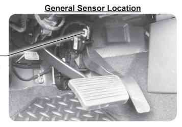
**STEP 10 -** Connect one end of the supplied harness to the sensor, and the other end to the factory harness. Secure the harness with the supplied zipties. Make sure none of the AMP'd components interfere with pedal operation.
