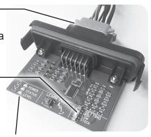
**STEP 15** - Turn the ignition on. The STATUS indicator should be flashing and the LEVEL indicator should be off.
