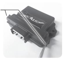
**STEP 12 -** Connect the circuit board—to the AMP'd harness. Keep away from metal objects that might cause a short circuit.
