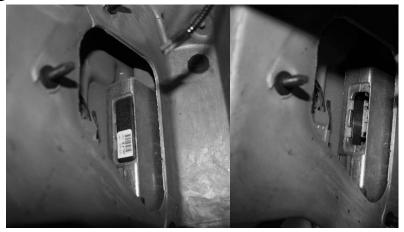
5 With the provided Scotch-Brite pad clean the rubberized protective coating off of the terminal contacts. Both sides of the terminal need to be cleaned. It is important that the contacts are sufficiently clean to avoid any connection issues.
