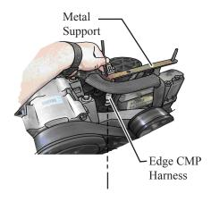
8. Once the CMP sensor is located, and the Edge harness plugged in, use zip ties to keep all parts of the harness away from the belt or other moving parts.
