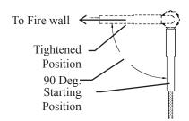
7. Make sure that the probe cable is positioned to allow best path and minimal bending for routing to the fire wall.
