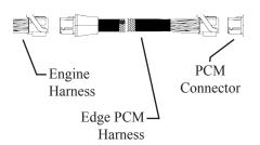
CAUTION: The two connectors should slide easily together. DO NOT force the two connectors together. If the connectors do not slide smoothly, inspect for bent pins, and retry.
