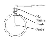
6. Install the probe into the fitting, and tighten the top nut of the fitting just tight enough to keep the probe firmly mounted.
