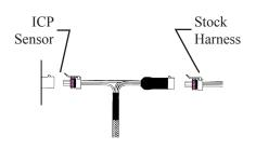
NOTE: The ICP connection is located in the middle of the engine compartment, and to the right of the MAT sensor (Towards driver side).
