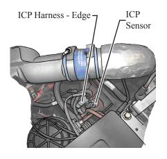
CAUTION: The ICP sensor closely resembles the coolant sensor which is located towards the front of the engine.
