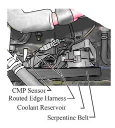
CMP ASSEMBLY (LOOKING "UP" FROM UNDERNEATH THE TRUCK)
