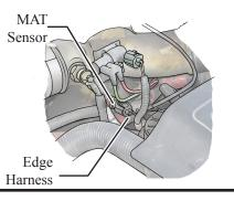
5. Connect the ICP connectors in between the stock harness and the sensor.
