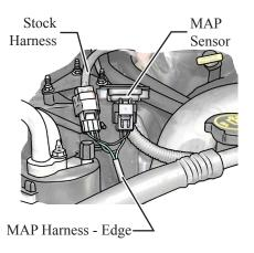
4. Connect the MAT connectors in between the stock harness and the sensor as shown.
