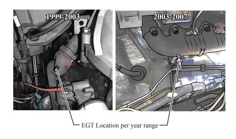
NOTE: Find these exhaust manifold locations by laying on your back behind the driver side front tire and looking up. The 1999-2003 view shows only the fitting having been installed. The 2003-2007 view shows the Probe mounted to the fitting.
