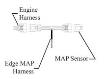
13. Use zip ties to fasten the harness. Keep all harness components away from hot engine surfaces, as well as moving parts.
