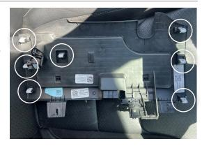
**STEP 4** - To make the CAN junction box more accessible, use a trim tool to carefully work around the 6 clips on the lighting switch panel. Once removed, set the panel aside.
