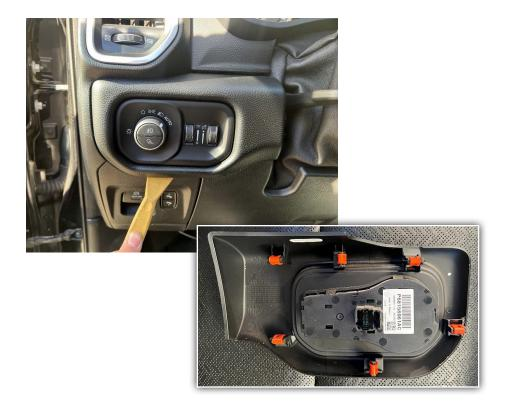
**STEP 5** - Route the CAN connector to the junction box located on the driver's side of the dashboard. Plug into any open port of the green junction box.
