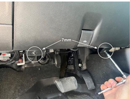
**STEP 3** - Pull the lower dash panel while out being careful not to break the plastic clips. See image for plastic clip locations.
