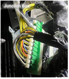
STEP 8 - Locate the Star Connector Junction Box under your dash above the Parking Brake Release Latch. Connect to the green junction box in ANY open port. NOTE: It is possible that the green junction box is covered or hidden by black fabric tape/material.
