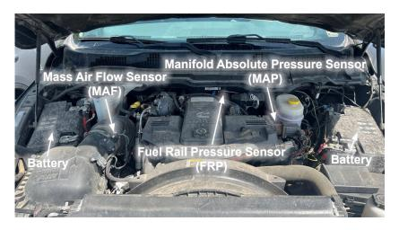
**STEP 2** - Locate the MAP Sensor on the driver side of the engine bay in front of the Brake Master Cylinder, and disconnect it by pushing in on the tab to release. Connect both connectors to the EZX harness.
