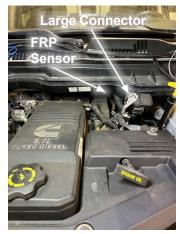
unlock the connector (**NOTE**: You may need to use needle nose pliers or a pick tool). Once released, press in directly on the lock tab as you pull to release the connector. Connect both connectors to the EZX harness.
