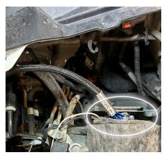
**STEP 11** - Use the provided zip ties to secure the excess cable from touching hot surfaces or any moving components.
