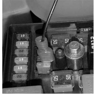
**STEP 4** - Connect the included 2-Blade Fuse Plug (A) to the Unlock Cable and plug the Fuse Plug into the slot you pulled the original fuse from. Ensure that you orient the Fuse Plug so that the wire is coming out on the side closest to the driver side of the vehicle, and furthest from the passenger side.
