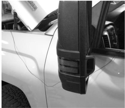
**STEP 5** - Route the Unlock Cable out of the engine bay, around the driver side A-Pillar, and through the open window.
