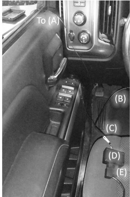
**STEP 7** - Plug the Unlock Cable (C) into the Locksmith module (D).
