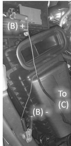
**STEP 6** - Route the rest of the Unlock Cable over to the vehicle's battery. Slide open the red (positive) battery terminal cover and clip the red (positive) Alligator Clip (B) from the Unlock Cable into the positive tab inside. Then, clip the black (negative) Alligator Clip (B) onto a nearby Ground stud.
