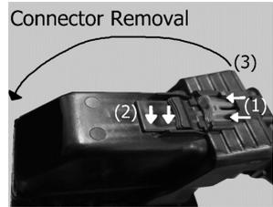
**STEP 4** - Open the locking lever (3) all the way and then the connector can be pulled off of the TCM. You can push the TCM connector aside and leave it dangling; it is on a short cable and will not drop further into the engine bay.
