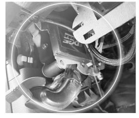
**STEP 12** - Use the provided zip ties to secure the excess cable from touching hot surfaces or any moving components.
