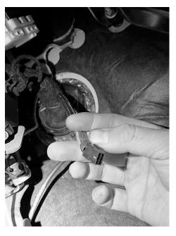
**STEP 8** - Reconnect the 6-pin Access Link connectors back together inside the cab.
