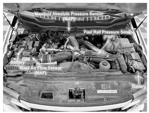
**STEP 2** - Locate the MAF connector on the intake box, and disconnect it by pulling the locking tab up then squeeze the release tab. Connect both connectors to the EZX harness.
