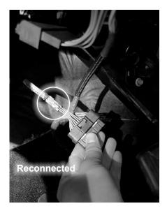
**STEP 9** - Locate the APP Sensor above the accelerator pedal and disconnect it by pulling up on the red locking tab and then pushing in the release tab. Connect both connectors to the EZX harness.
