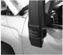
**STEP 4** - Route the Unlock Cable out of the engine bay, around the driver side A-Pillar, and through the open window.
