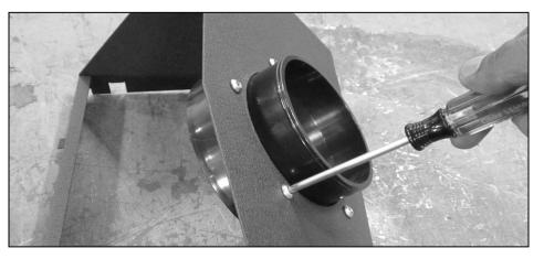
**STEP 9** - Mount your Jammer air filter to the adaptor installed in step 8 with the clamp provided
