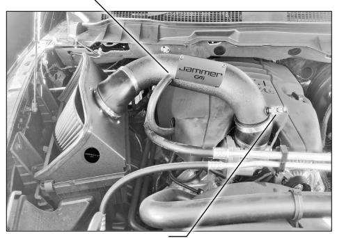
STEP 17 - Connect the temperature sensor harness.
