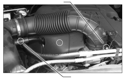
STEP 4 - Disconnect the crank case line from the air box.
