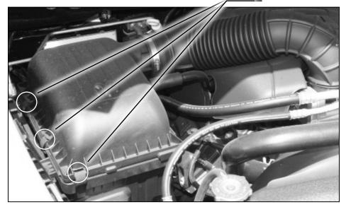
STEP 2 - Disconnect the Temperature Sensor harness from factory intake.
