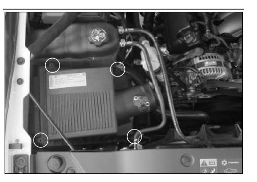
**STEP 7 -** Remove the top portion of the stock intake housing by removing the 4 factory screws. Retain for later use.
