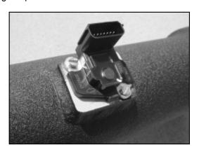
**STEP 11 -** Install the trim seal on the edge of the top corners of the Jammer housing.
