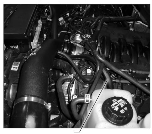
**STEP 15 -** Replace the stock crankcase vent tubes with the supplied hoses.
