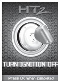
**STEP 5** - Allow the device to search for DTCs to clear.
