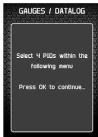
**STEP 5** - Select a PID Group, then select a total of 4 PIDs. Use the ◀ / ▶ arrows to switch between screens. OK to select.
