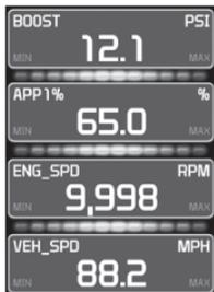
**STEP 2** - Press the OK button to begin recording the PID data. Press the OK button again, to stop the recording.
