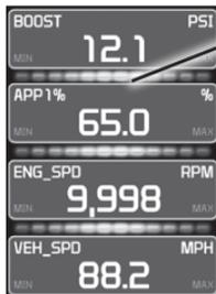
The separator lines will change from Red to **Green**, which indicates that the device is actively **recording** (datalogging).
