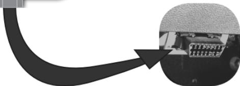
**STEP 1** - Plug the device into the OBDII port.
