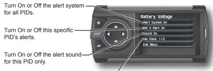
This is the point at which you want the alert to be triggered for this PID. The example above shows 11.5 as the value. If the display detects a battery voltage of 11.5 volts or less, the alert will be triggered.
