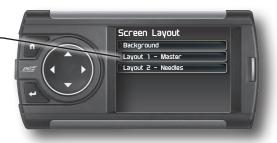
STEP 4 - Use the Up/Down buttons to scroll through the available screen layouts. Press Enter to select an option.
