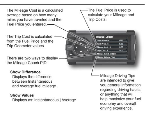
**STEP 4** - Refer to the Individual Gauge Set Up section of this manual to display one or both Mileage Coach PIDs on the main gauge screen.
