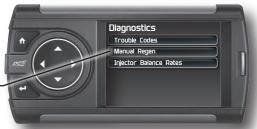
NOTE: When manually initiating a regeneration cycle, some vehicles will require a drive cycle (i.e. you have to drive the vehicle some distance) while others may allow you to initate a Service Regeneration where you can leave the vehicle parked and the engine running. If the latter is the case, be sure to use the following guidelines.
