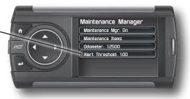
**STEP 6** - Use the Up/Down arrow buttons to adjust the threshold value.
