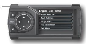
STEP 4 - Use the Up/Down arrow buttons to highlight a new PID, then press Enter.
