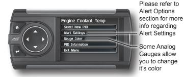
**STEP 6** - Return to the main gauge screen. The new PID will be displayed along with any customized options you may have changed.
