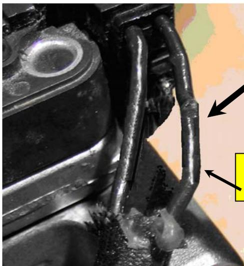
**NOTE:** *Important-while the connector halves are being seated together the wire is not to be rotated. The stock wiring harness that plugs into the injection pump may be disconnected for better access to the wire.*
