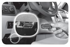
1. Plug the HT into the OBDII port.
