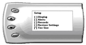
The *Evolution* has the ability to correct for changes in tire size. If you have changed your tires to a different size the PCM will miscalculate vehicle speed which can affect shifting as well as the speedometer. Correcting the tire size will allow the Evolution to accurately calculate vehicle speed. **You will need to enter in a tire size, if you would like to display MPH.** To change your tire size, two formats are available for you to use; you will only need to choose one format.
