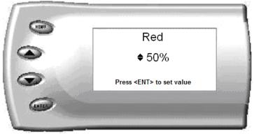
6. As you adjust the percentage shown on the screen, you should notice a change in the color of the screen. Once the desired color value has been reached, press [ENTER]. If you would like to return to the previous screen and abort the current color change, press [MENU].
