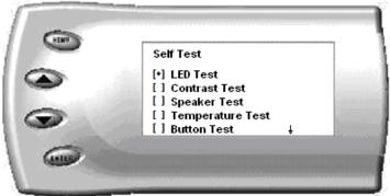
After the test is complete, press [MENU] repeatedly to return to the *Diagnostics* and *Main* Menu Screens.
