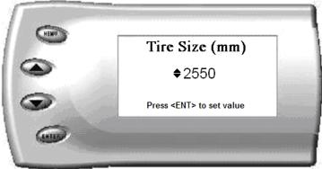
The numbers on this screen represent the circumference (in mm) of your tire size. The default value the *Evolution* displays is the current value stored in the PCM. Adjust the tire size by pressing the [UP] and [DOWN] arrow keys.
