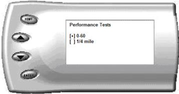
3. Select the desired performance test (0-60 screen is shown below). If your vehicle is moving at this time, the *Evolution* will ask you to come to a stop.
