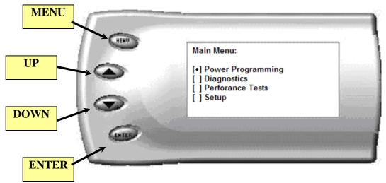
**NOTE:** The Evolution uses a LCD display which has inherent limitations in operating temperature. If your screen is black, blank, or distorted and the temperature is above 158 degrees F (70 degrees C), please allow the device to cool and then it should work correctly. At extreme low temperatures (32 degrees F, or 0 degrees C) the display will update very slowly. Again wait for the device to warm to normal operating temperatures for the screen to function properly.
