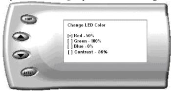
4. Select *Contrast*, and use the up and down arrows to adjust the contrast to where you'd like.
