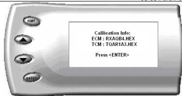
This screen shows the calibration info of the truck that the *Evolution* is currently connected to.
