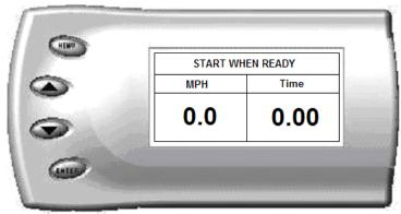
4. For the 0-60 MPH run, press the accelerator pedal and the test automatically begins. For the ¼ mile test, you will be asked to press a key when ready. It will then cycle through a starting light sequence (Christmas tree) and tells you when to go. As you drive, the screen
