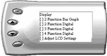
3. Select the style which you would like the parameters to be displayed on your screen and press [ENTER]. Depending on which display you select, a screen similar to the following appears:
