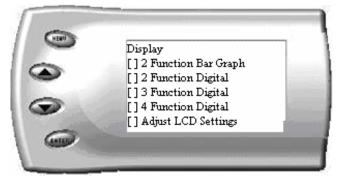
3. Select the desired viewing option by using the [UP] and [DOWN] arrows and pressing the [ENTER] key on the desired display type.
