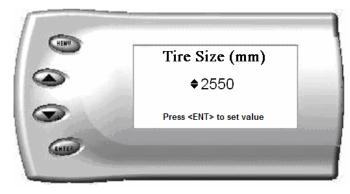
The numbers on this screen represent the circumference (in mm) of your tire size. The default value the *Evolution* displays is the current value stored in the PCM. Adjust the tire size by pressing the [UP] and [DOWN] arrow keys.
