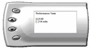
3. Select the desired performance test (0-60 screen is shown below). If your vehicle is moving at this time, the *Evolution* will ask you to come to a stop.
