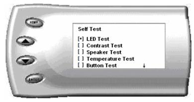
After the test is complete, press [MENU] repeatedly to return to the *Diagnostics* and *Main* Menu Screens.
