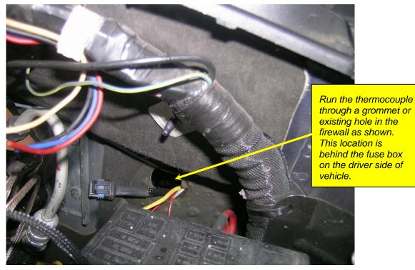
4. Run the cable up under the dash and secure it with the supplied Zip ties. After the supplied OBDII connector cable is installed, you will connect the end of the thermocouple cable to the port on the right side of the OBDII connector as shown in following picture.
