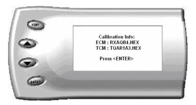
This screen shows the calibration info of the truck that the *Evolution* is currently connected to.
