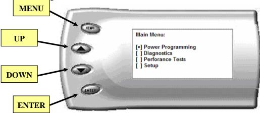
**NOTE:** The Evolution uses a LCD display which has inherent limitations in operating temperature. If your screen is black, blank, or distorted and the temperature is above 158 degrees F (70 degrees C), please allow the device to cool and then it should work correctly. At extreme low temperatures (32 degrees F, or 0 degrees C) the display will update very slowly. Again wait for the device to warm to normal operating temperatures for the screen to function properly.
