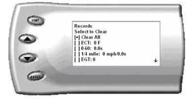
3. This is where you can view all of the current recorded high values. The arrow located at the bottom right corner of the screen indicates there are more parameters than the display can show. Use the [UP] and [DOWN] arrow keys to scroll through the list of records. If you would like to reset a single parameter, select the desired parameter and press [ENTER]. If you would like to reset all of the records, select the *Clear All* option and press [ENTER]. To exit out of this list press [MENU].
