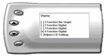
3. Select the style which you would like the parameters to be displayed on your screen and press [ENTER]. Depending on which display you select, a screen similar to the following appears:
