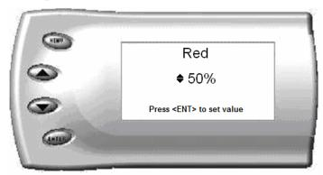
6. As you adjust the percentage shown on the screen, you should notice a change in the color of the screen. Once the desired color value has been reached, press [ENTER]. If you would like to return to the previous screen and abort the current color change, press [MENU].
