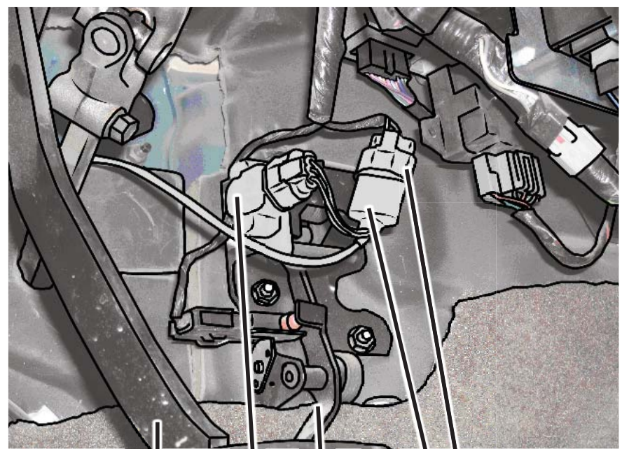
Brake Linkage TPS Sensor Accelerator Linkage Truck Harness TPS Adapter - Edge
