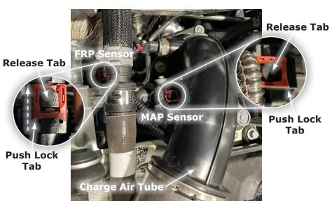
**STEP 11** - Move the Pulsar XT harness up under the windshield tray so that they are not pinched underneath the Charge Pipe or Intake Tube.
