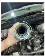
NOTE - To remove the Spring Clip, push the charge tube in towards the cab. Then, pull on both sides until they click into their respective latches. The Spring Clip should then unlock, freeing the Charge Pipe.
