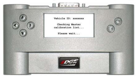
2. The *Evolution* will check the PCM and determine if it is in the Master Calibration list. If the calibration is available, you will see the following message:
