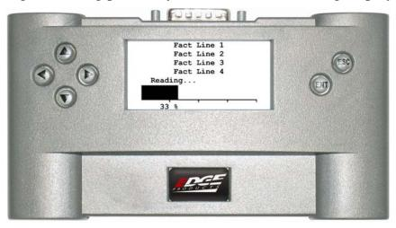
4. If this is the first time the unit is used on a particular vehicle, the *Evolution* will build and verify the modified calibrations (Skip to step 5 for subsequent programming operations). During this process, you will see the following displays:
