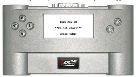
14. After pressing <ENT>, the *Evolution* tests the PCM for communications. If successful, a truck does a "Burnout" and the FINISHED screen appears:
