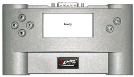
When you press the accelerator pedal, the test automatically begins. As you drive, the screen should be displaying your current speed. When the test is complete (the desired distance or speed is reached), the test will automatically stop and your result will be displayed on the screen.
