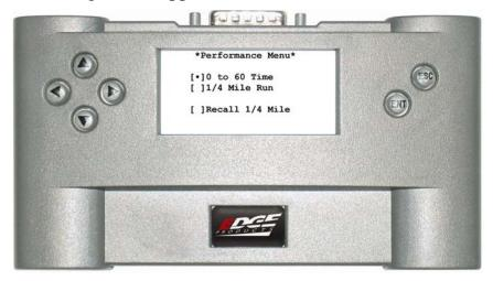
3. Select the desired performance test and press <ENT>. If your vehicle is moving at this time, the following screen appears:
