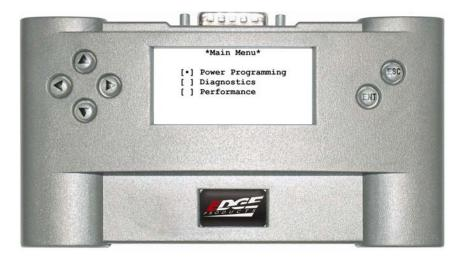
2. Select your desired option by pressing the up or down keys on the left side of the programmer and press <ENT>. Continue to the next section.
